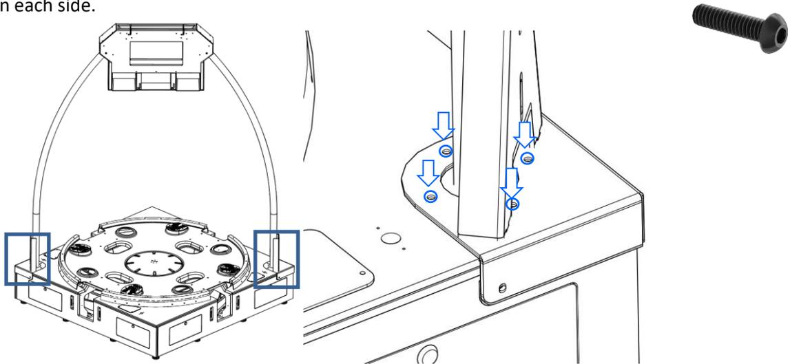
Secure each corner with the provided 2” button head screws and the ¼-20 locknuts
